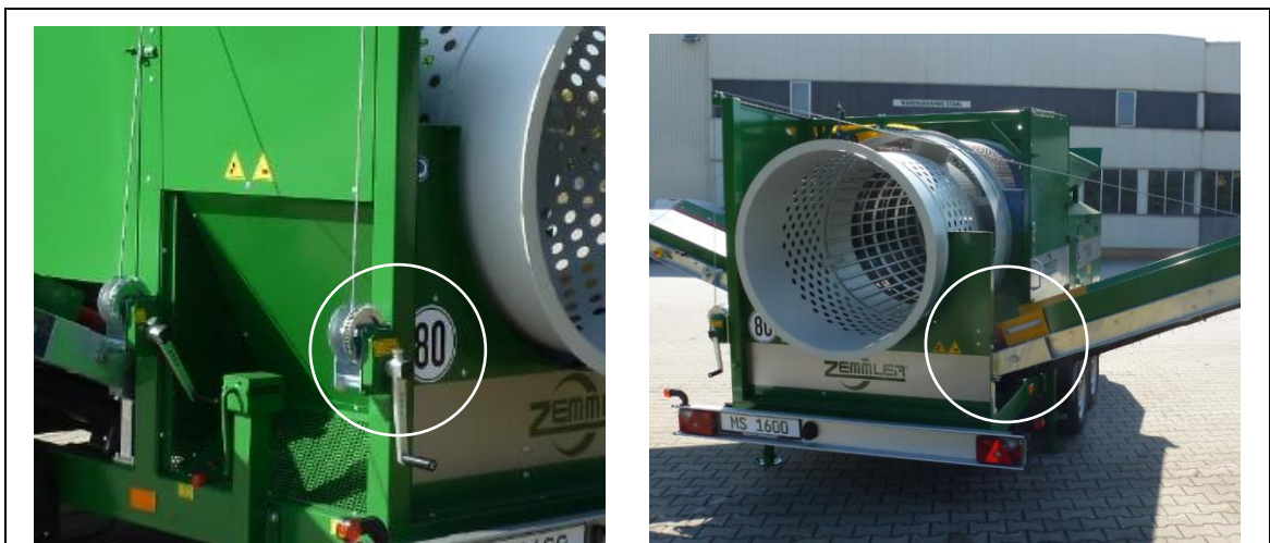
fig. 8-2: Coarse fraction with guide plates
