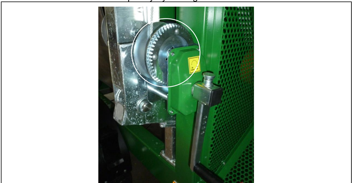
fig. 8-1: Crank/ rope winch of fine fraction
