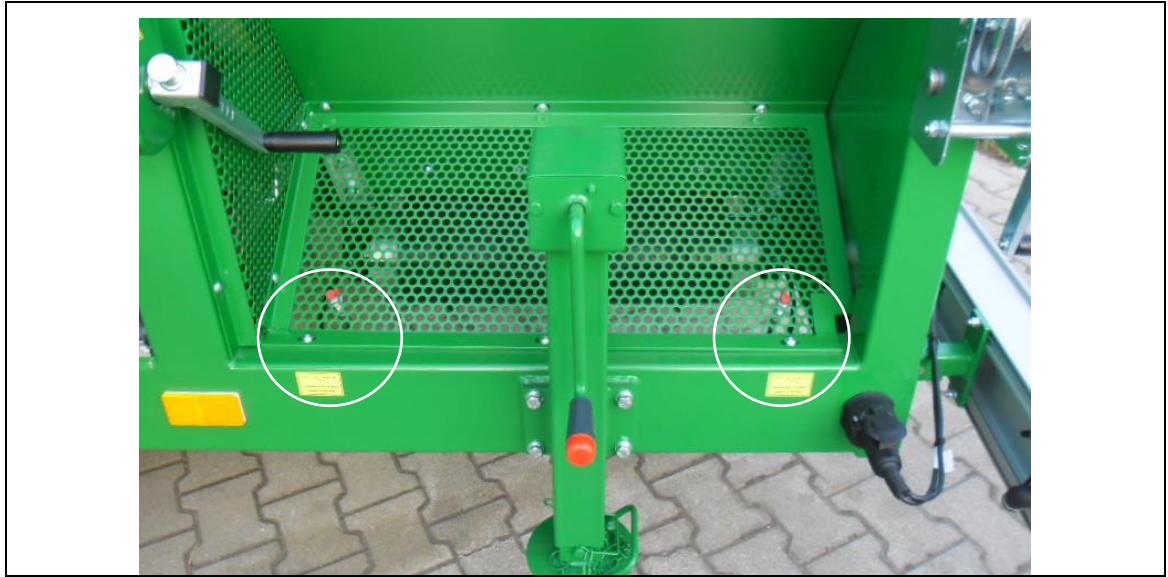
fig. 11-7: Lubrication points of coarse fraction
