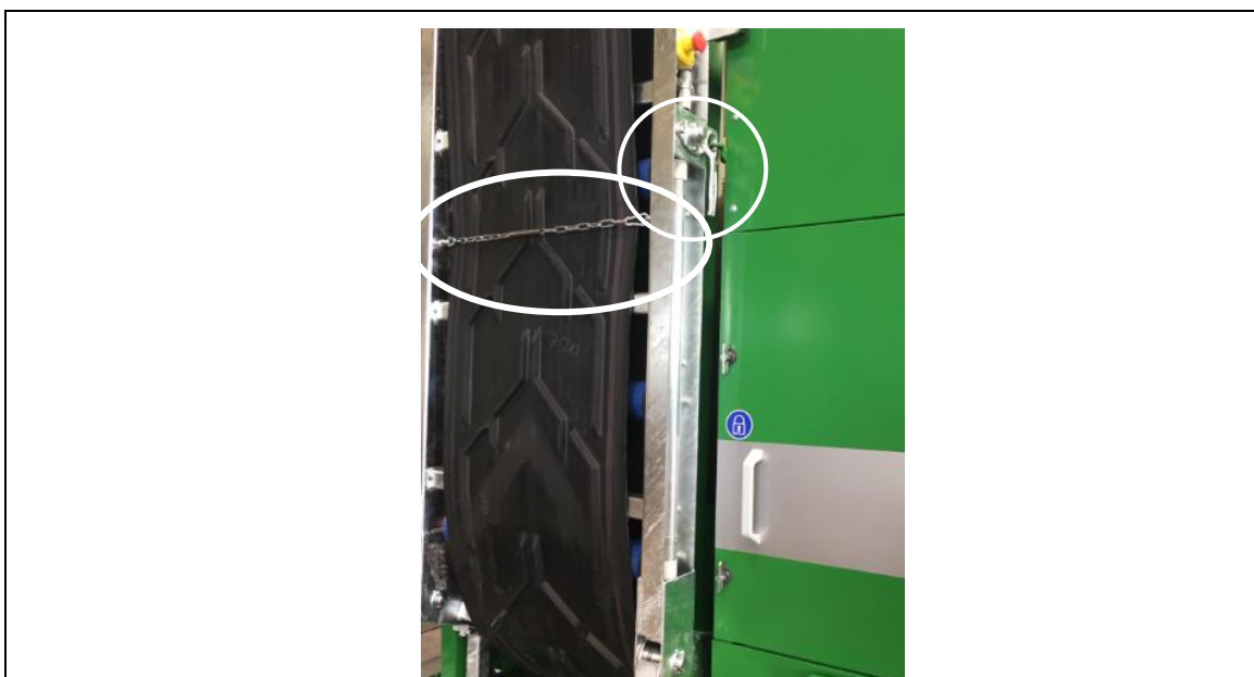
fig. 7-3: Transportation safety device of coarse fraction
