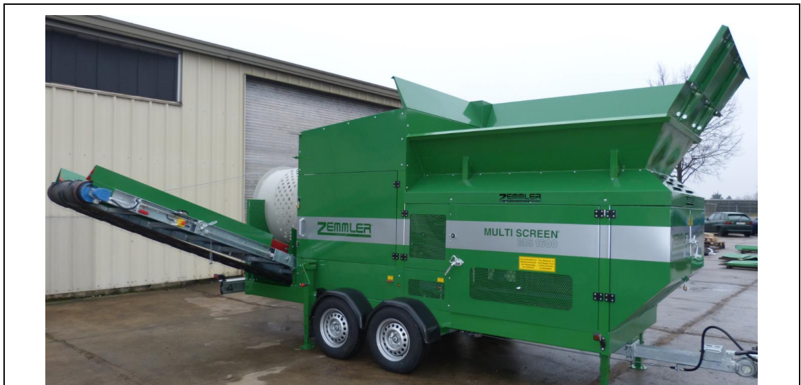
fig. 11-9: Mounted extension for 3 rd fraction and extended feeding hopper
