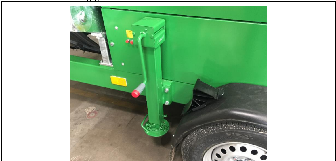
fig. 7-1: Landing gear in transportation position
