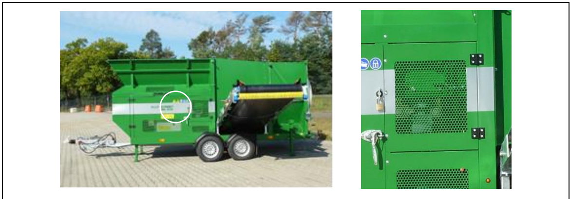
fig. 3-3: Cover protection and protection elements
