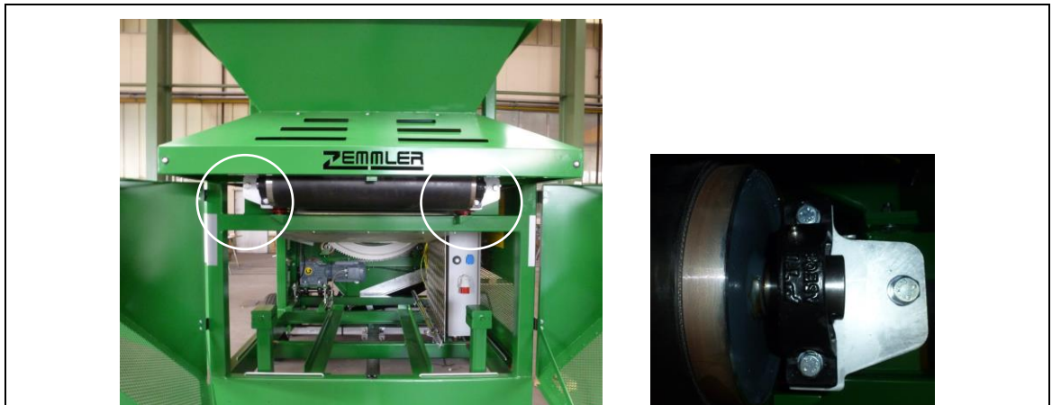
fig. 11-8: Lubrication points of feeder conveyor belt
