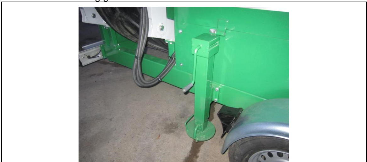
fig. 7-1: Landing gear in transportation position
