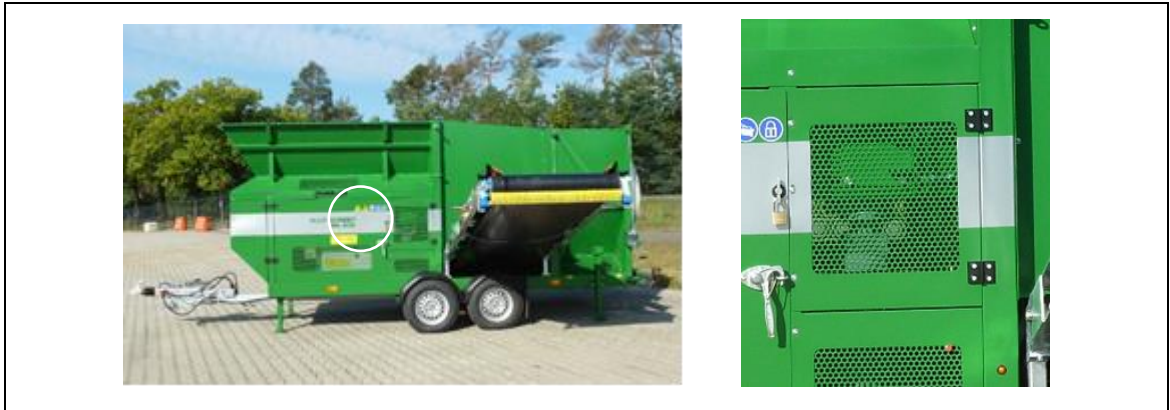
fig. 3-3: Cover protection and protection elements
