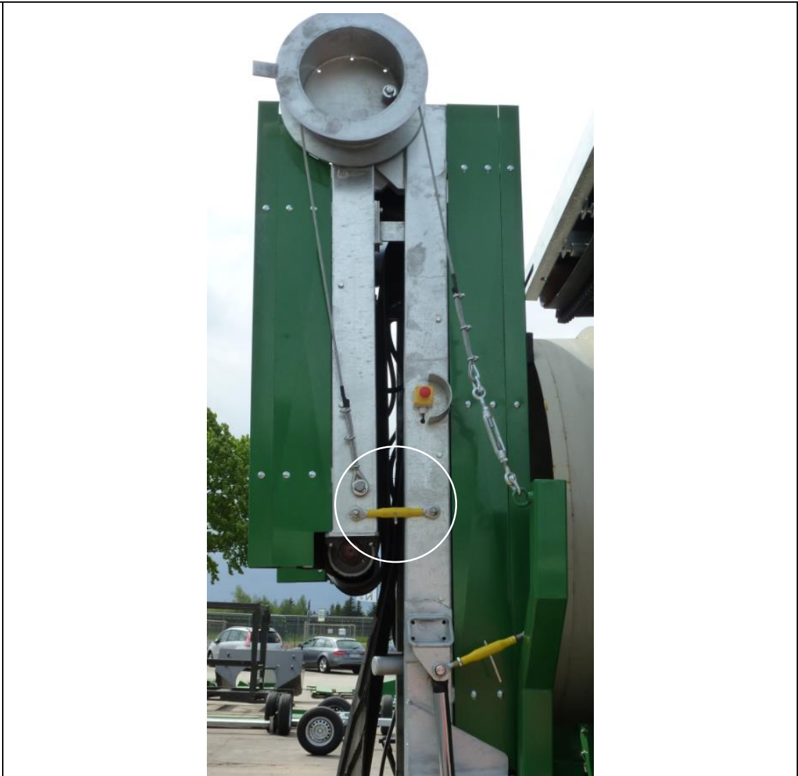
fig. 7-7: Transportation safety device of extended coarse fraction
