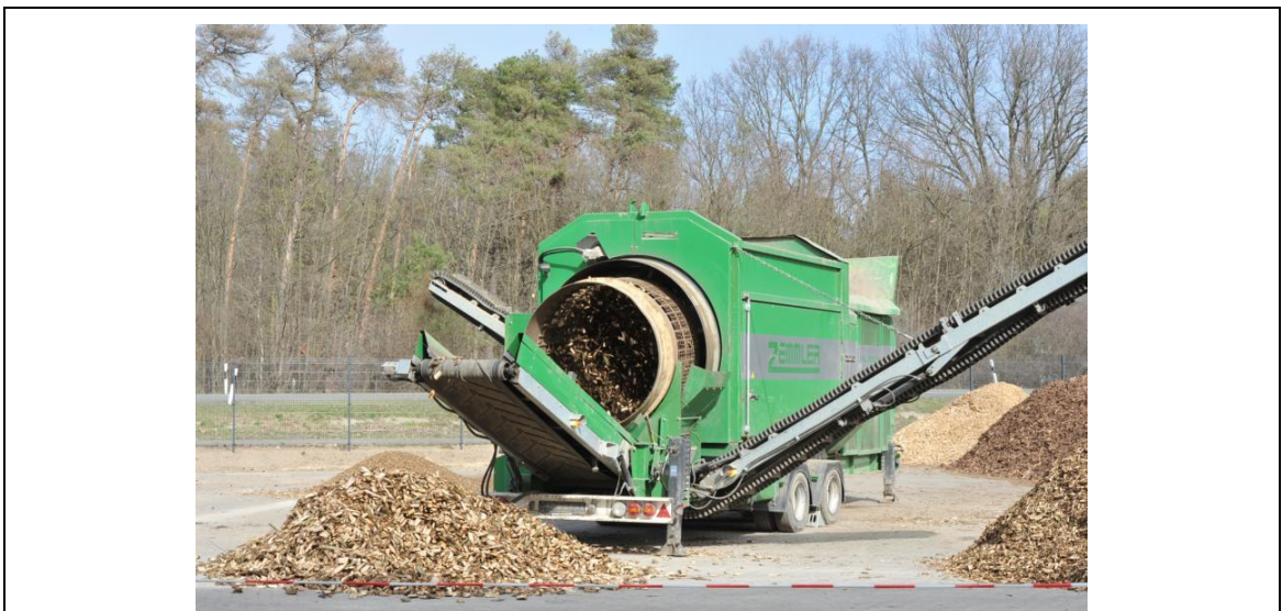
fig. 6-2: Example of double trommel in working mode (back right)
