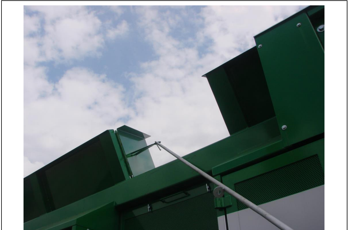
fig. 8-7: Hook rod and eye of the service door
