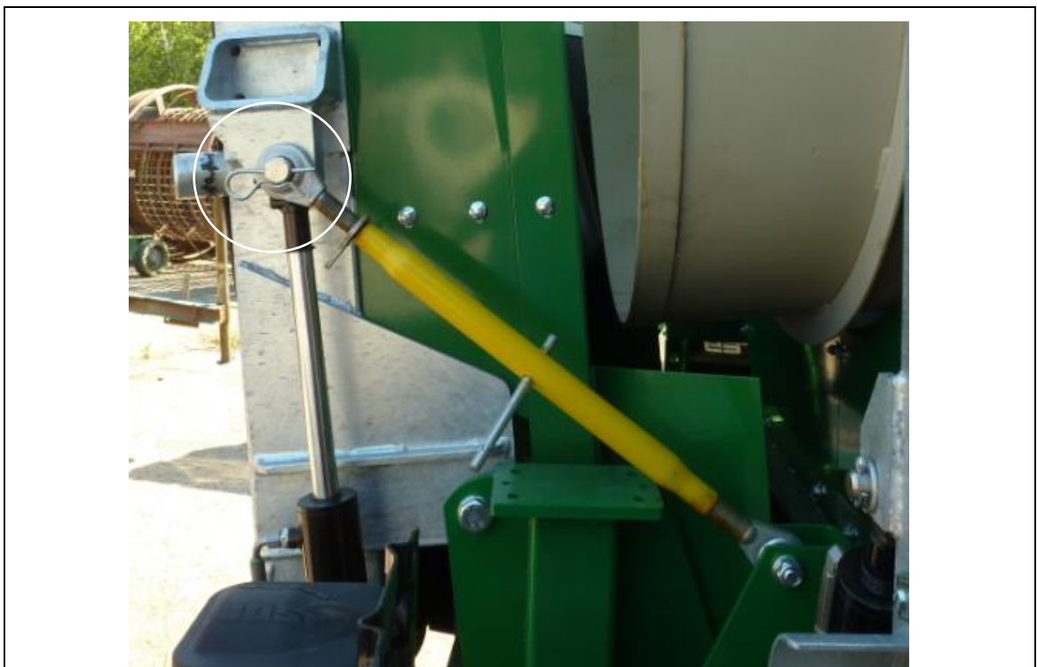
fig. 7-6: Transportation safety device of coarse fraction
