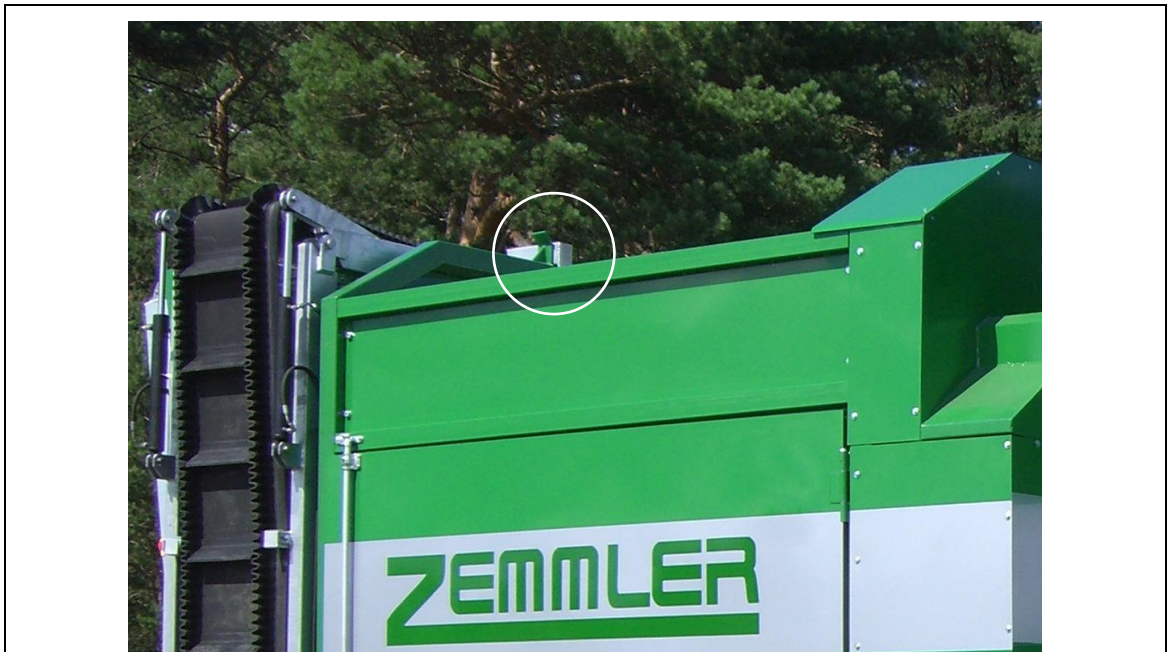
fig. 7-5: Transportation safety device of extended middle fraction
