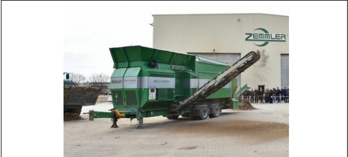
fig. 6-1: Example of double trommel in working mode (front left)
