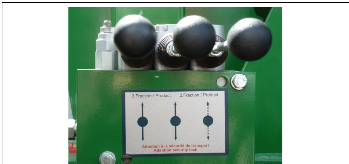
fig. 8-5: Control lever of extended middle fraction
