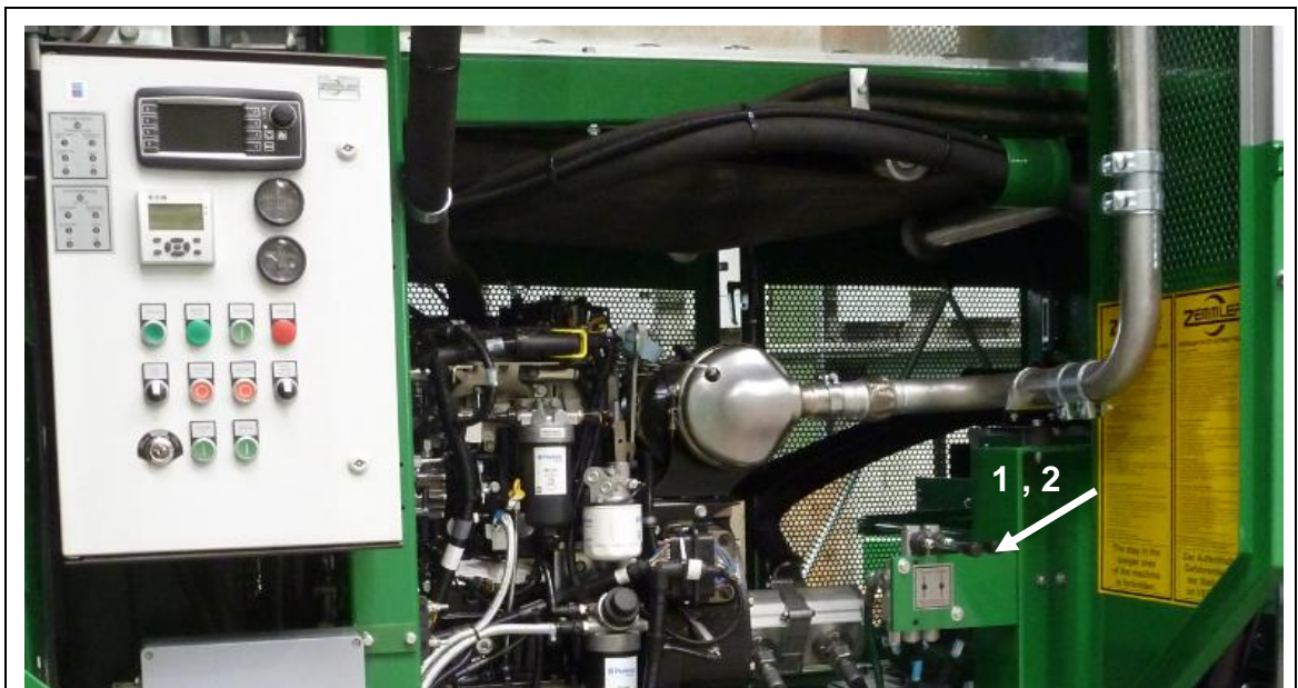
fig. 8-3: Control lever of fine fraction
