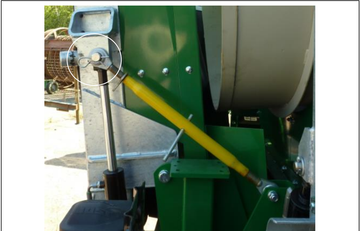
fig. 7-6: Transportation safety device of coarse fraction
