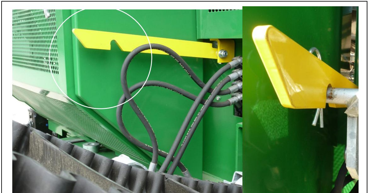
fig. 7-3: Transportation safety device of fine fraction
