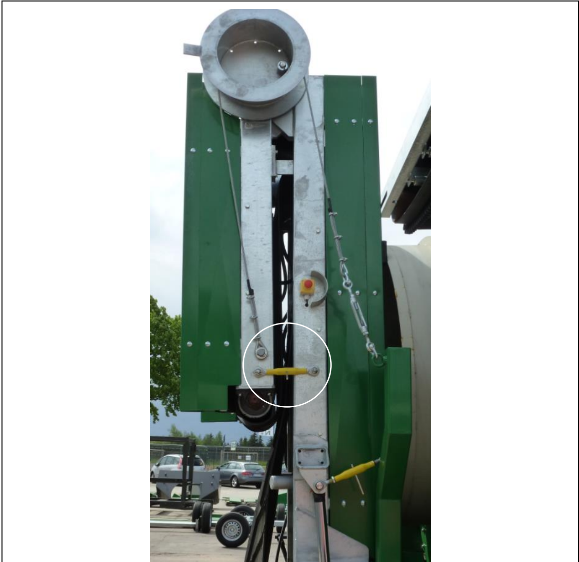
fig. 7-7: Transportation safety device of extended coarse fraction
