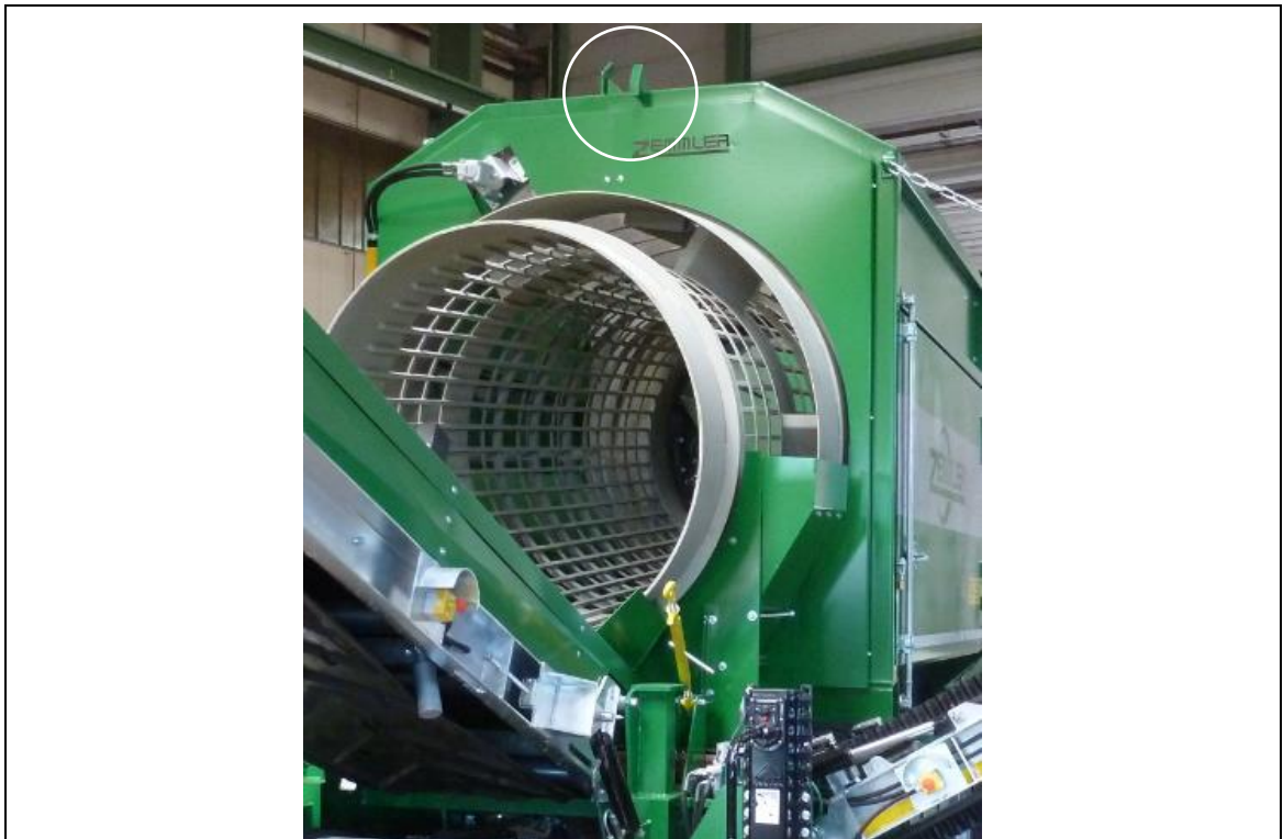
fig. 7-5: Transportation safety device of extended middle fraction
