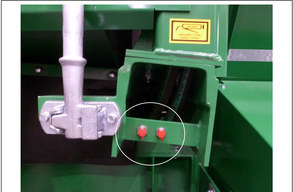
fig. 11-3: Position of grease points
