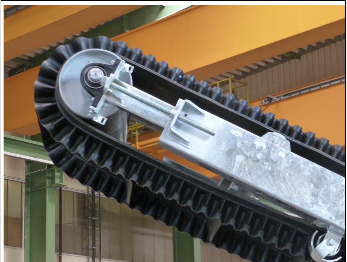
fig. 8-10: Upper adjustment fine and medium fractions in case of strip expansion
