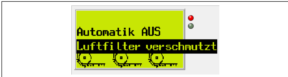
fig. 11-7: Monitoring of the air filter contaminated
