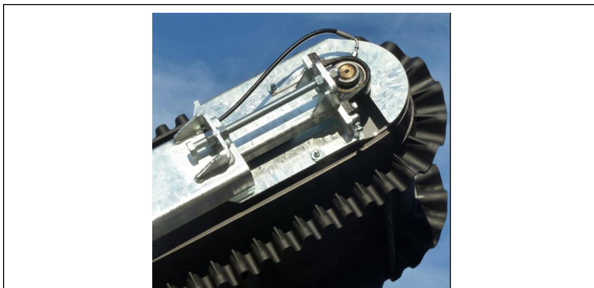
fig. 8-10: Upper adjustment fine and medium fractions in case of strip expansion
