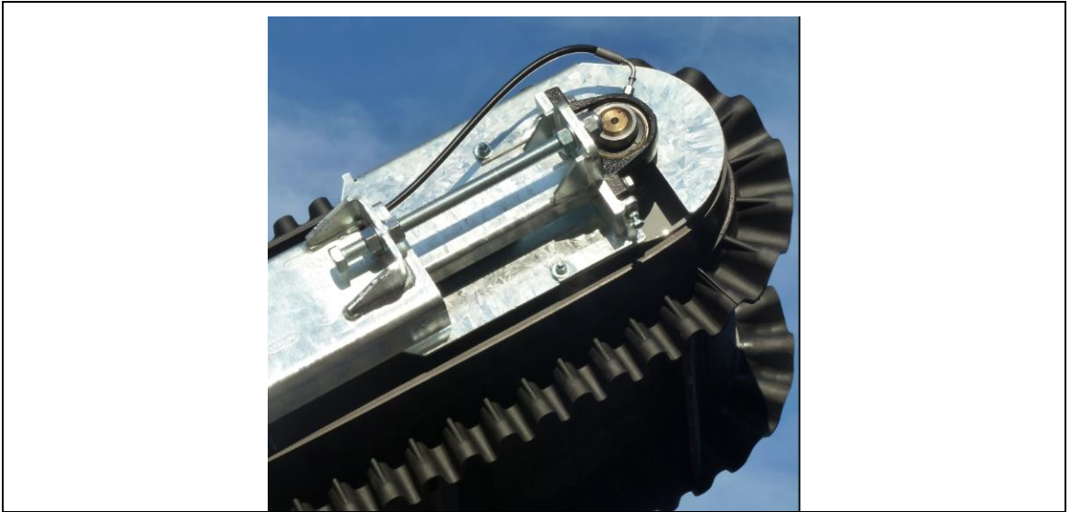
fig. 8-10: Upper adjustment fine and medium fractions in case of strip expansion
