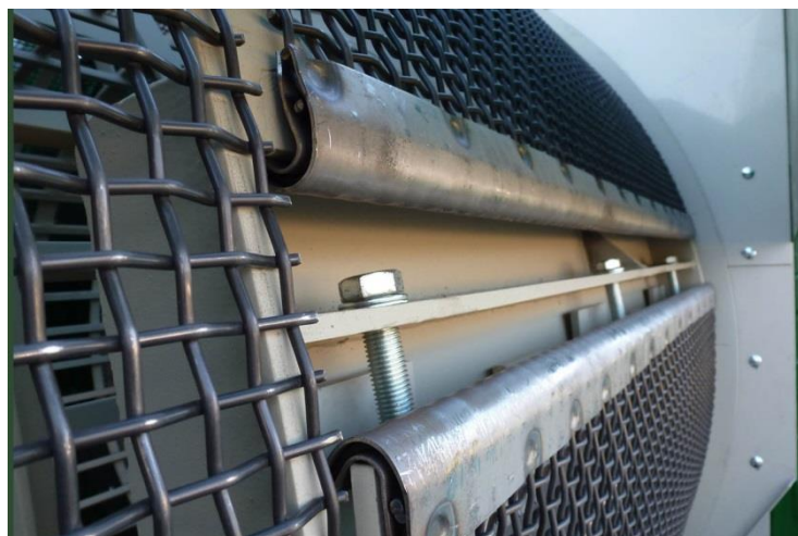
Fig. 11.2: Station de tension
