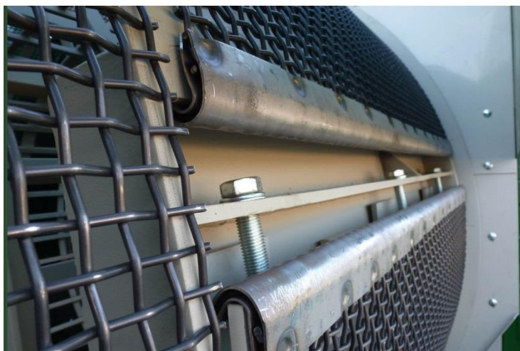
Fig. 11.2: Station de tension
