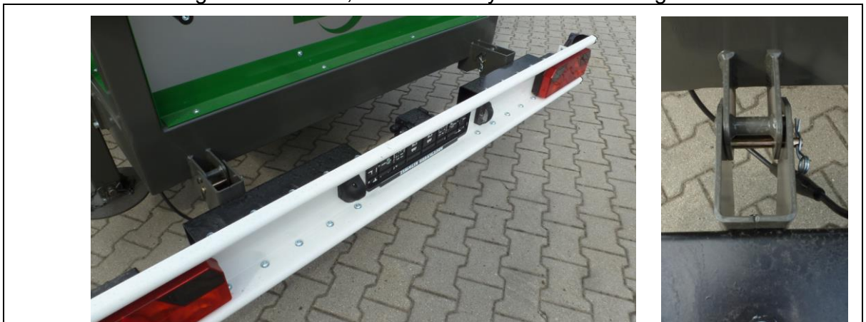
Fig. 7-3: Disconnect the fuse unit and the power supply to the light bar
