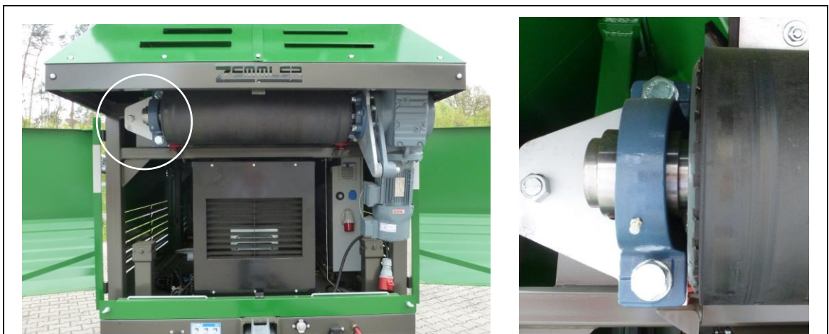
Fig. 11-10: Position of the lubrication points on the belt feeder
