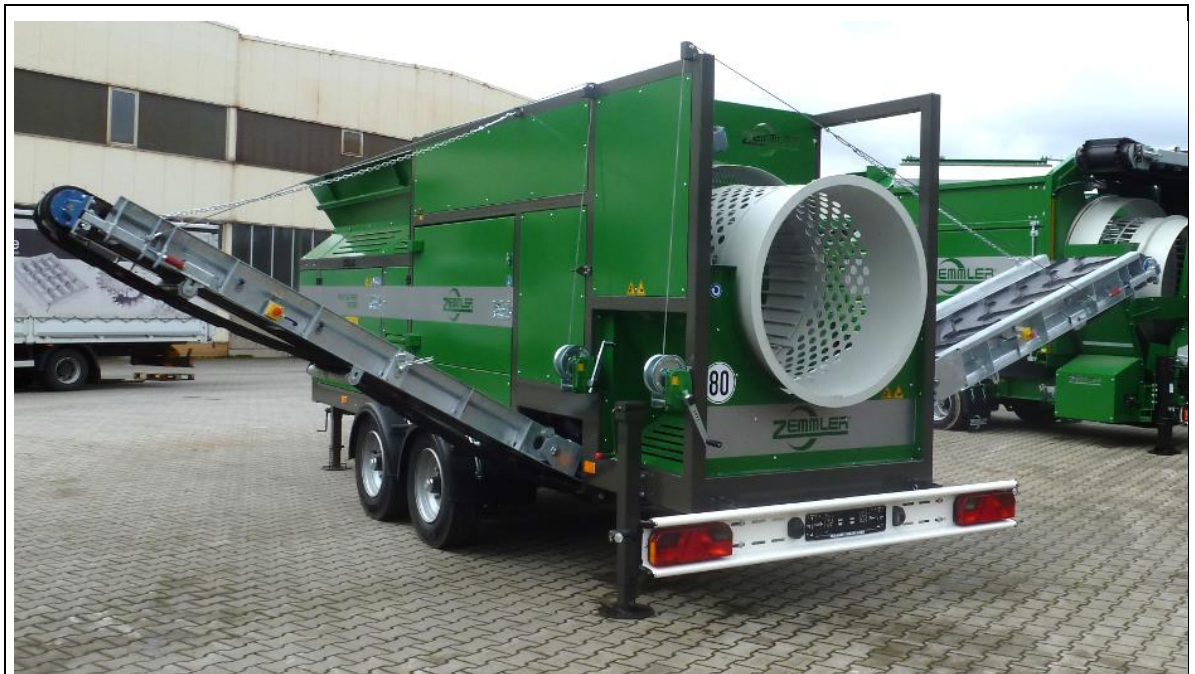
Fig. 6-2: Example of a screening system in working position (view from rear left)
