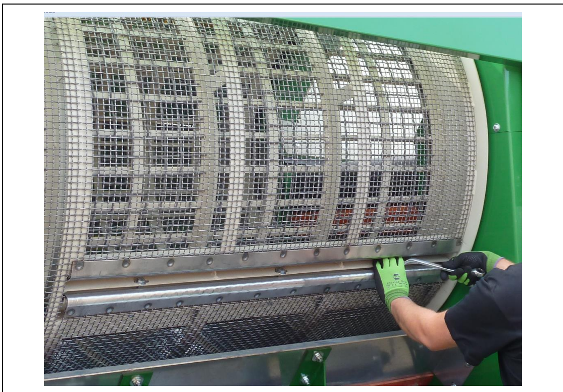
Fig. 11-3: Tensioning and fastening device for screen mesh covering (example)
