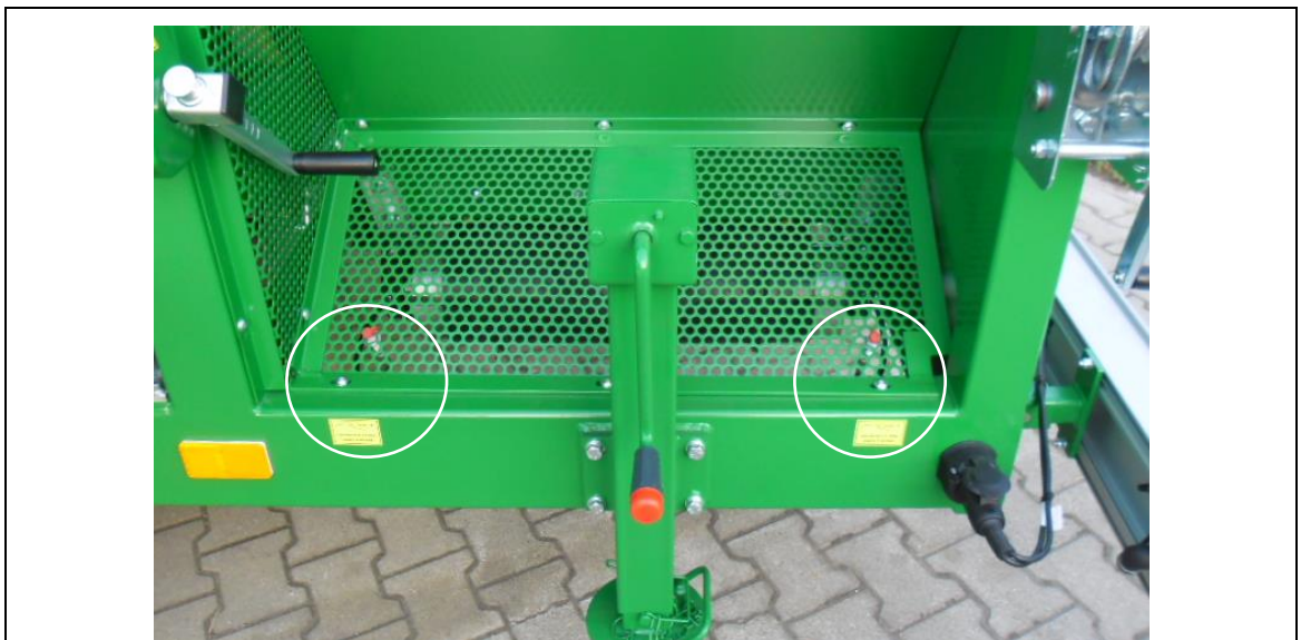
fig. 11-7: Lubrication points of coarse fraction
