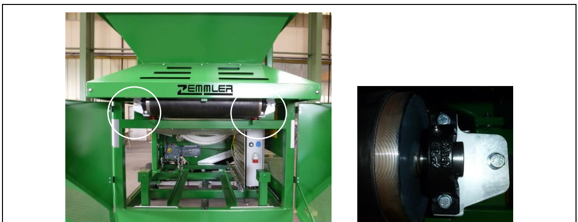
fig. 11-8: Lubrication points of feeder conveyor belt
