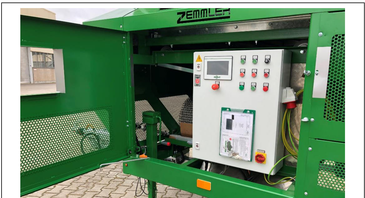
fig. 8-4: Control unit door opened
