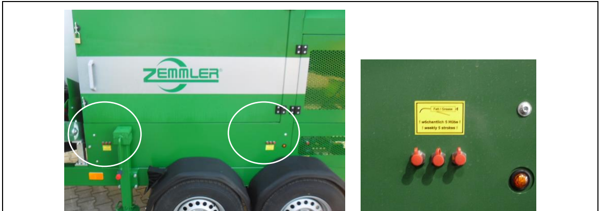
fig. 11-6: Lubrication points of fine fraction
