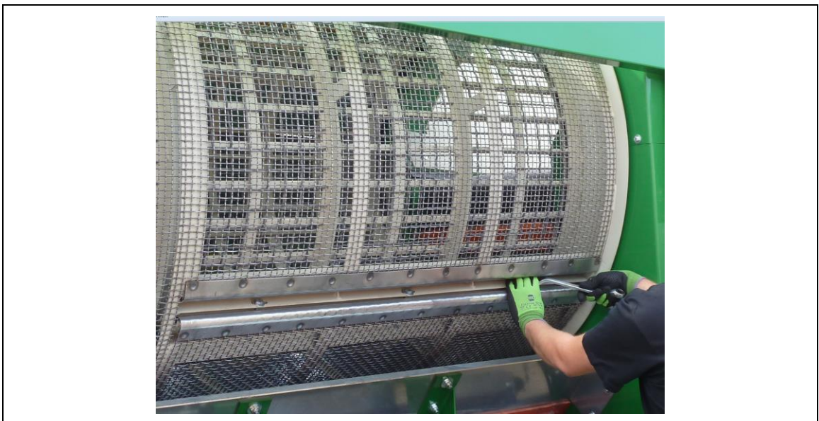
Figure 7-4: Tensioning and fastening device for screen mesh lining (example)
