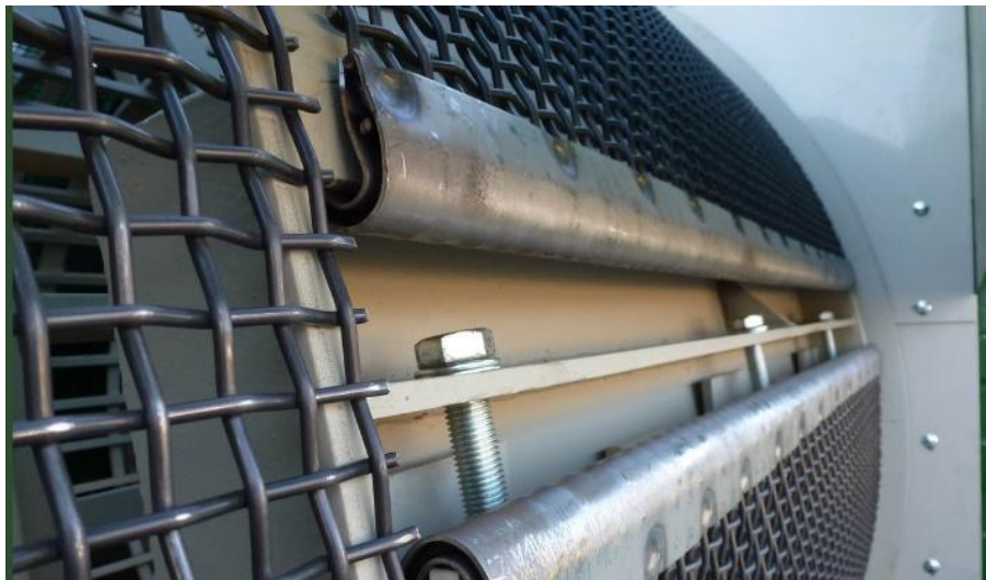
Figure 83: Clamping elements and screw connection via clamping station
