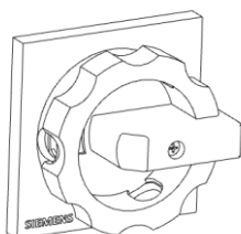
Figure 5: Main switch in the "OFF" position
