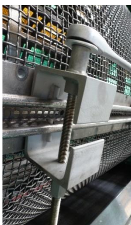
Figure 84: Tensioning the screens with a tensioning aid
