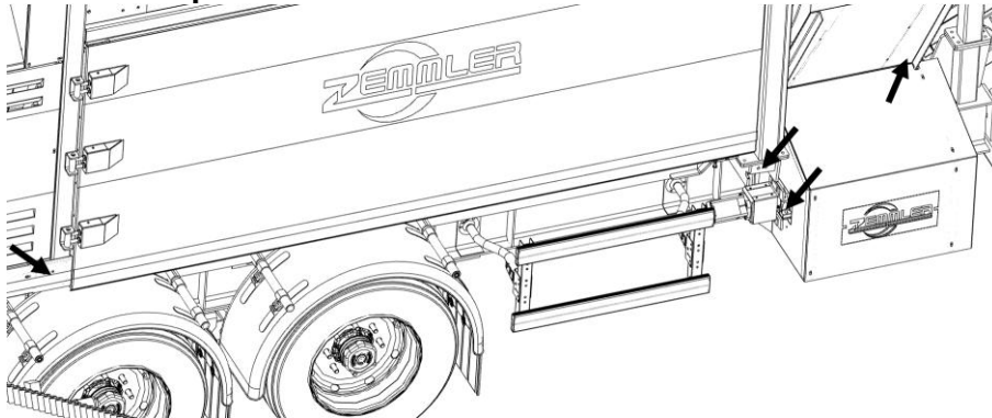
Figure 97: Position lubrication points housing left (31,32,33,37,38,41,42)
