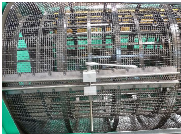
Figure 84: Tensioning the screens with a tensioning aid
