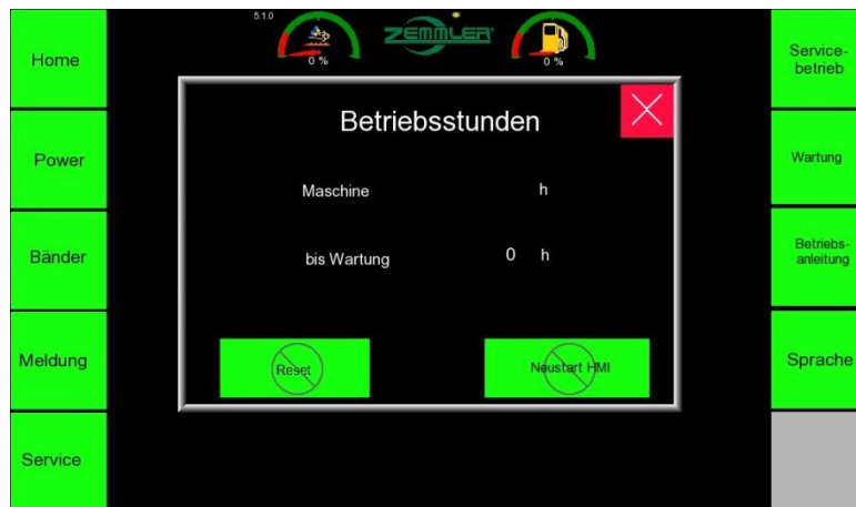
Figure 24: Screen display Operating hours
