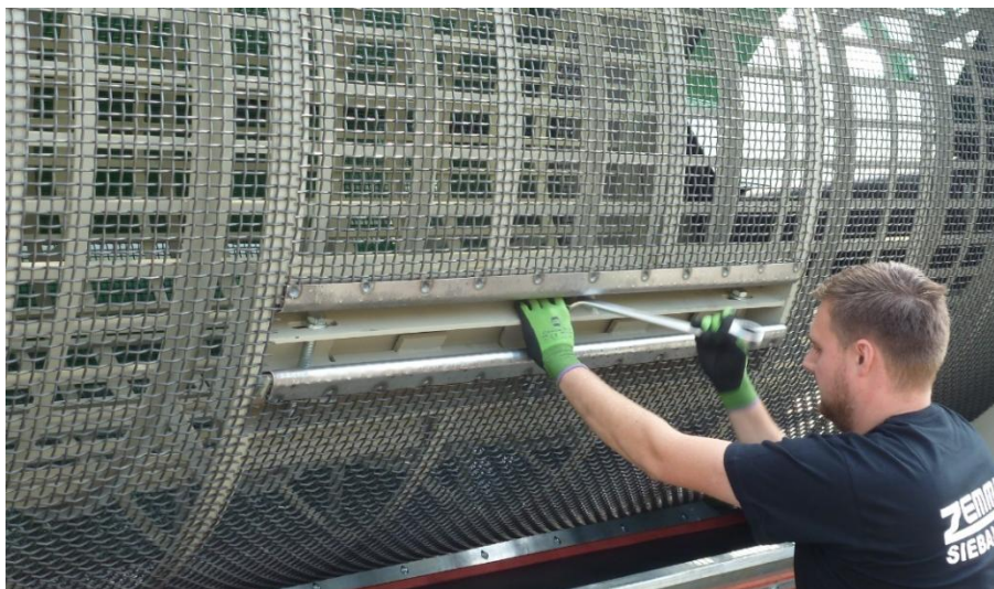
Figure 82: Tensioning the screens with tensioning station
