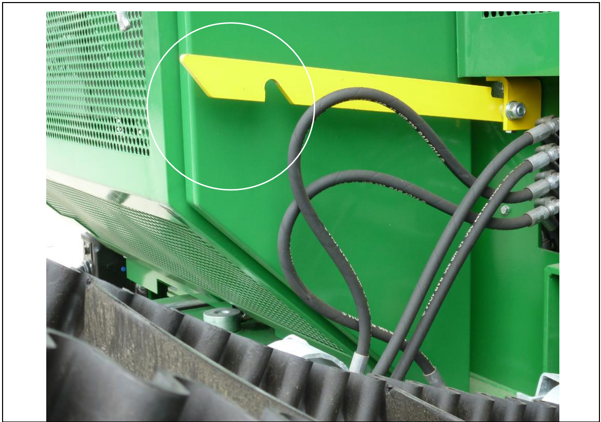
fig. 7-3: Transportation safety device of fine fraction
