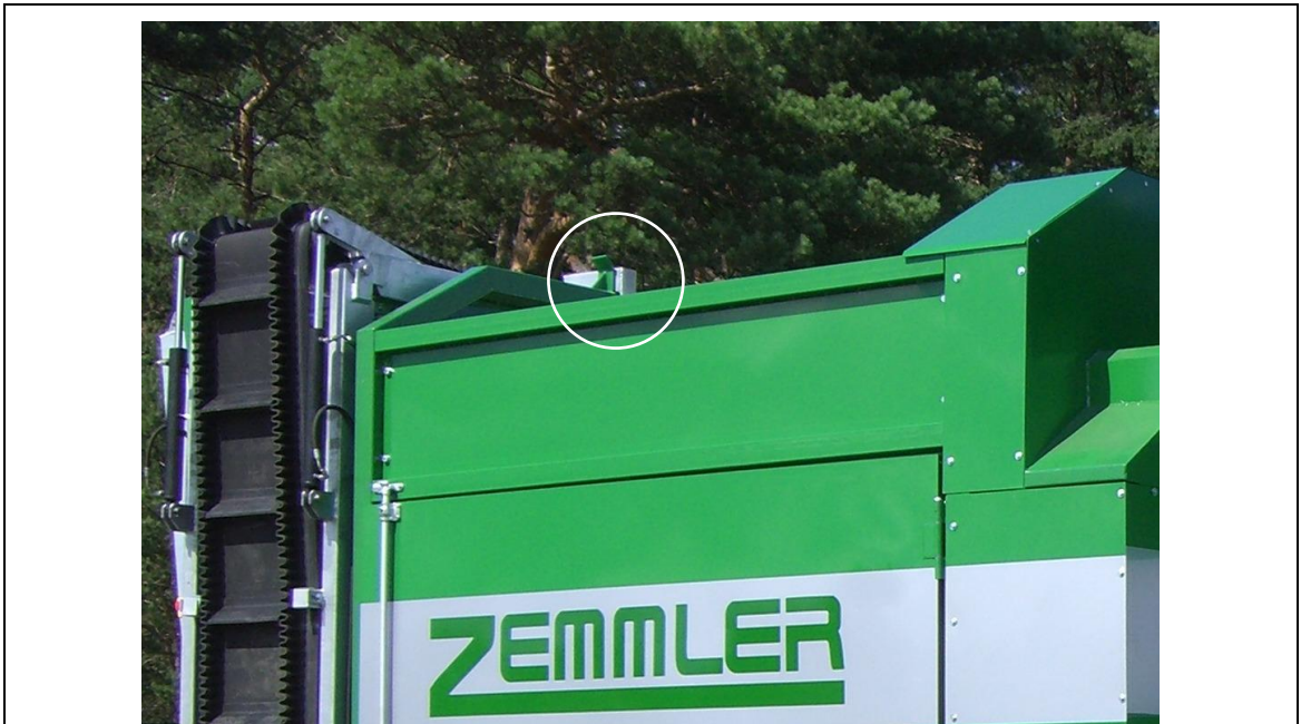
fig. 7-5: Transportation safety device of extended middle fraction
