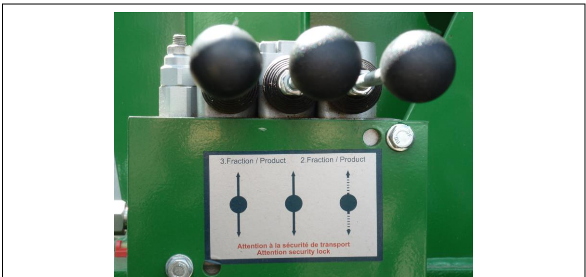
fig. 8-5: Control lever of extend middle fraction
