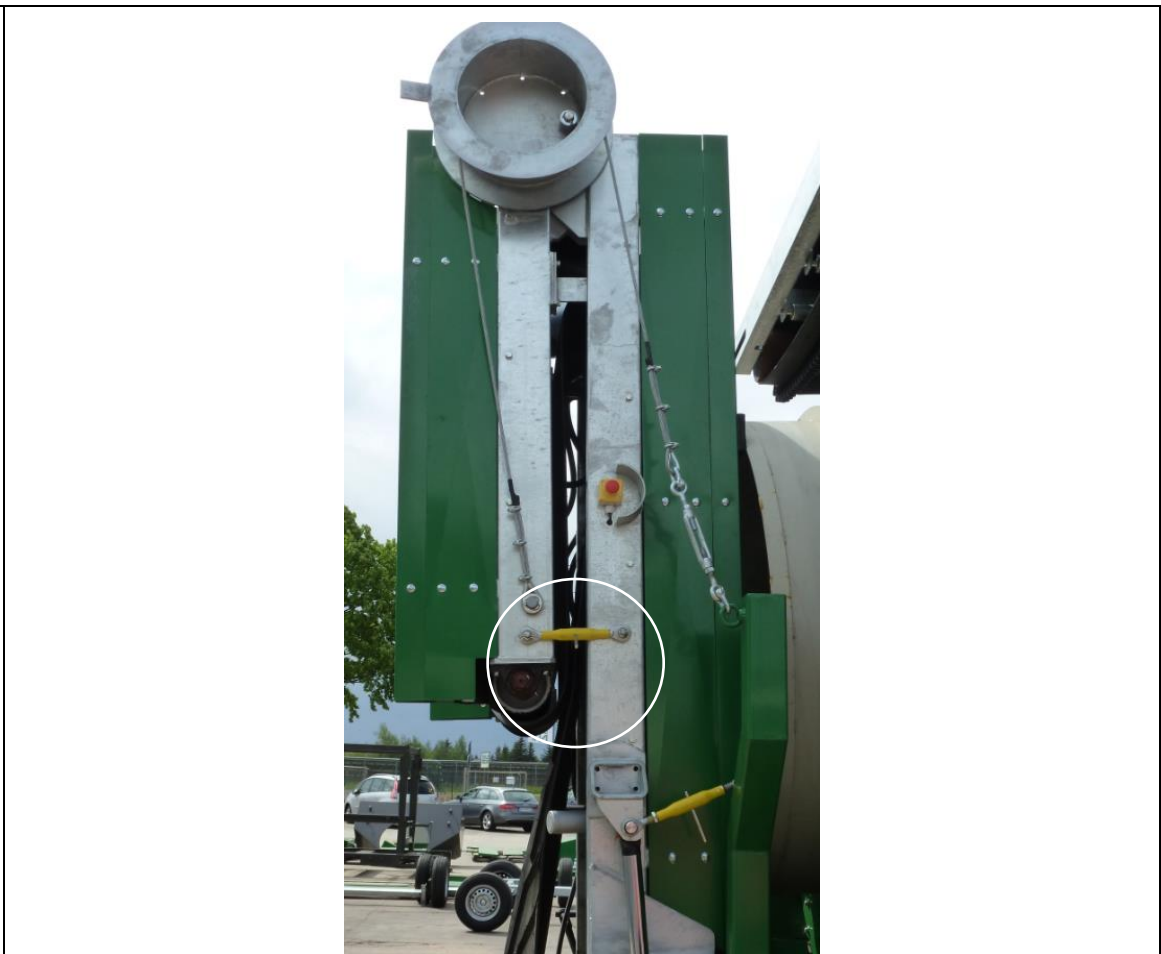
fig. 7-7: Transportation safety device of extended coarse fraction
