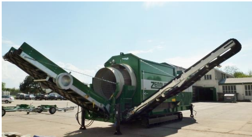
fig. 6-2: Example of double trommel in working mode (back right)
