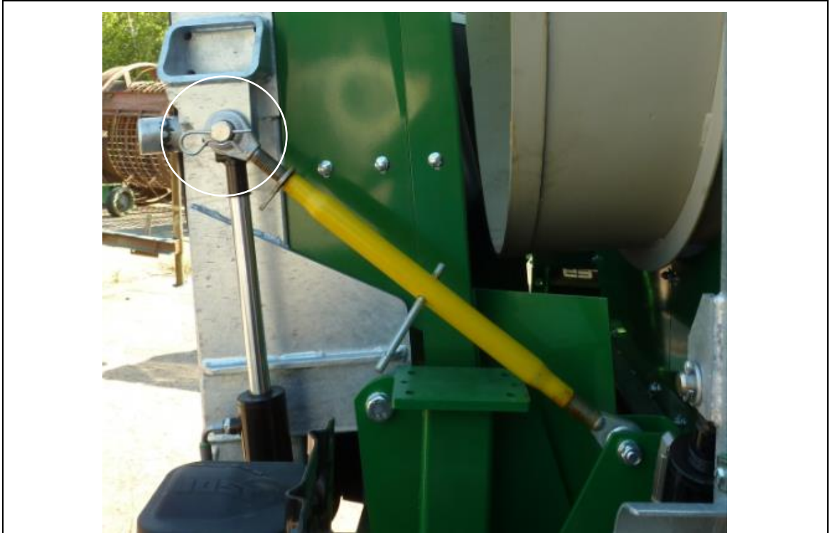
fig. 7-6: Transportation safety device of coarse fraction
