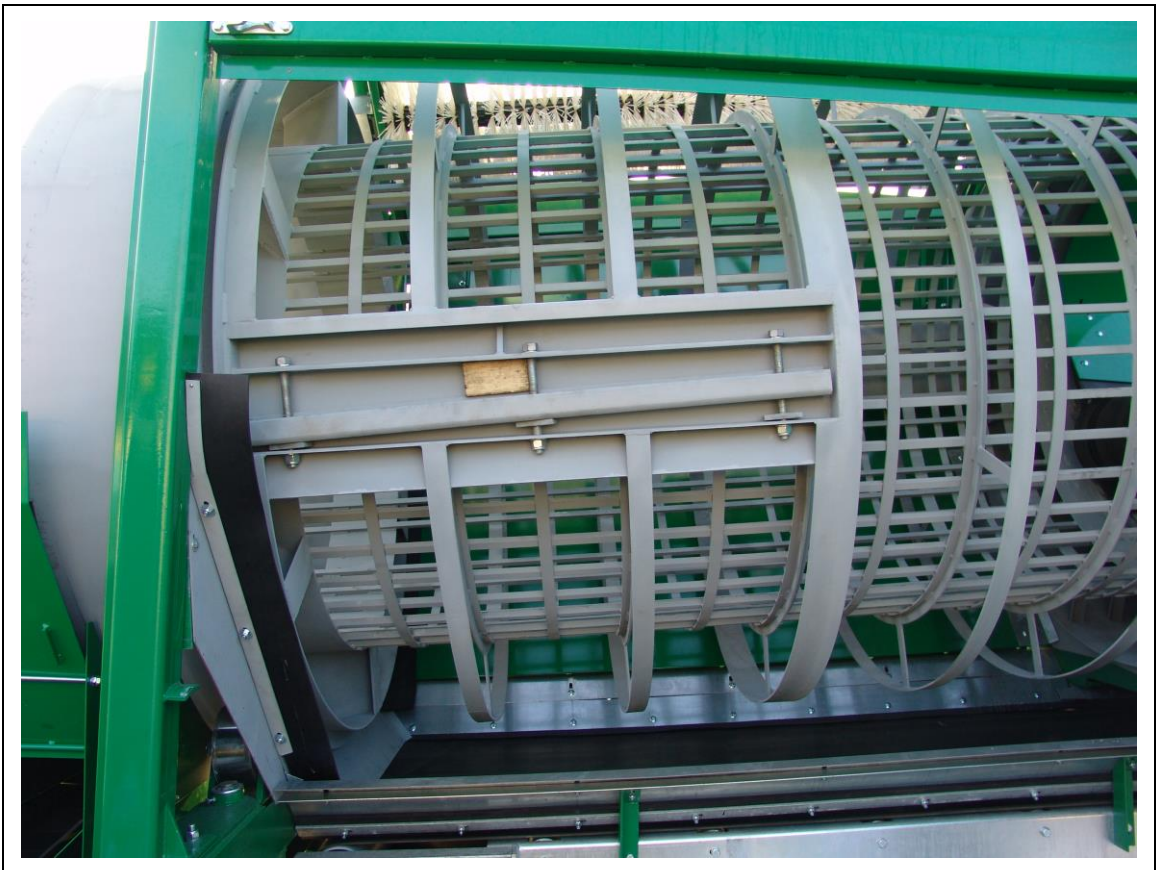
fig. 11-2: Clamping and fastening devices for wire screen pads
